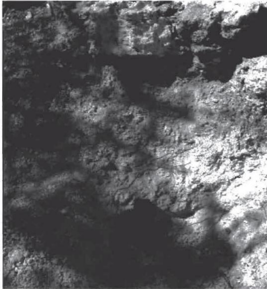
Figure 7. Nodular calcrete in a friable matrix under a 50 cm hardpan.
