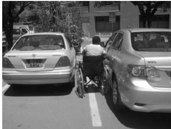
Figure 24: No space to transfer from or into the car
