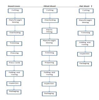
Fig 4 the process steps for Duvet Covers, Fitted Sheets, Flat Sheets
