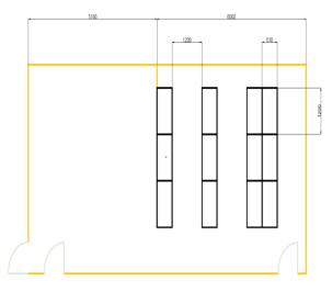
Fig 10 Recommended layout for the Finished Product storage section
