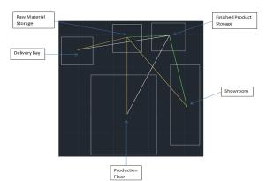
Fig 9 Alternative Space Relationship diagram with the finished product and raw material storage swapping locations
