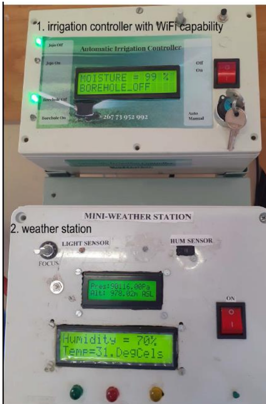
Figure 4.1(b): A working prototype of the Automatic Irrigation Controller undergoing tests.
