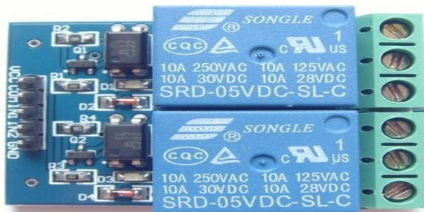
Figure 3.18: Two channel, 5V Relay Module [33].
