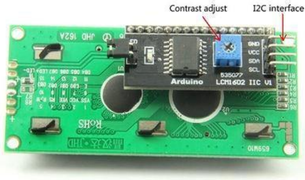
Figure 3.14: I 2 C interface bus to the 1602 LCD [29]
