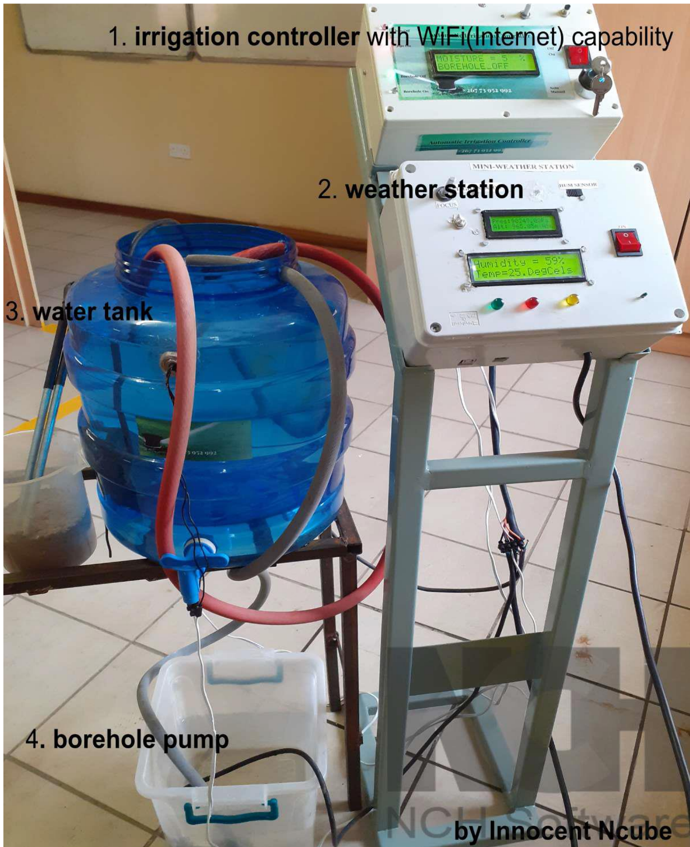
Figure 4.1 (a): The prototype undergoing laboratory tests
