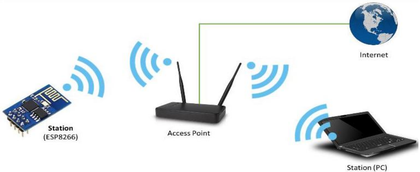
Figure 3.7: ESP8266 Wi-Fi board operating in the Station mode [22]
