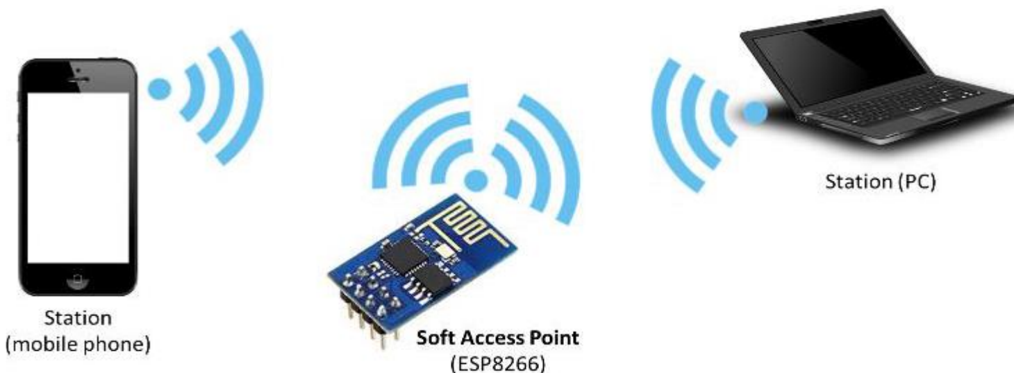
Figure 3.6: ESP8266 Wi-Fi module operating in the soft Access Point mode [22]
