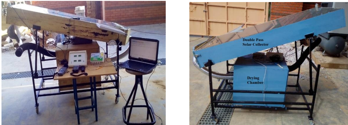
Figure 6. 1 Setting up and recording of parameters and final developed solar dryer.
