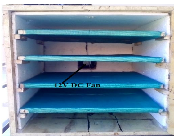
Figure 4. 2 Photographs showing experimental set up of the system and internal view of drying chamber.
