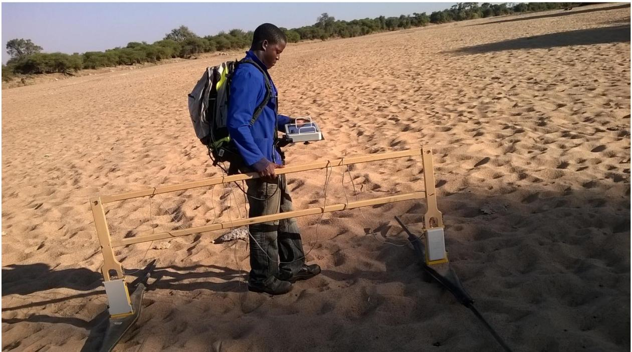
Figure 14: Display monitor, storage and control units and the antennae used for the survey
