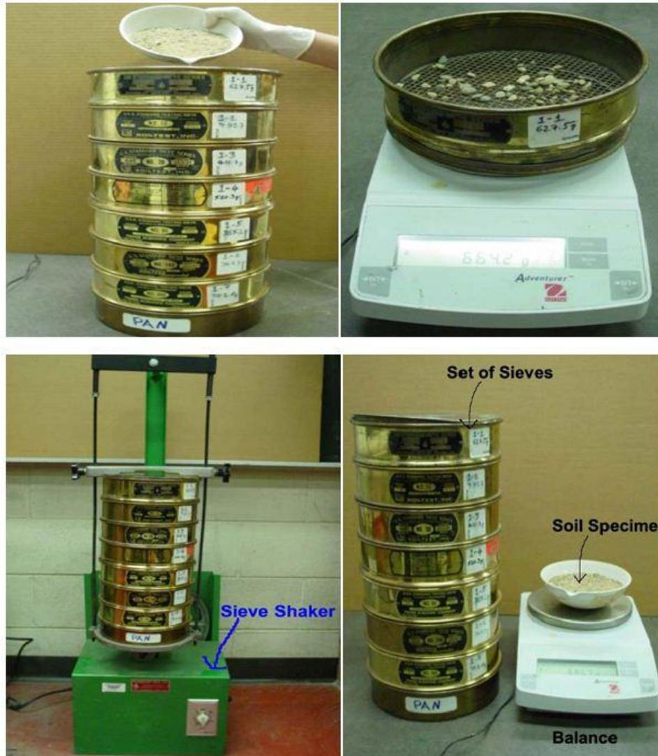
Figure 18: Equipment used for gradation
