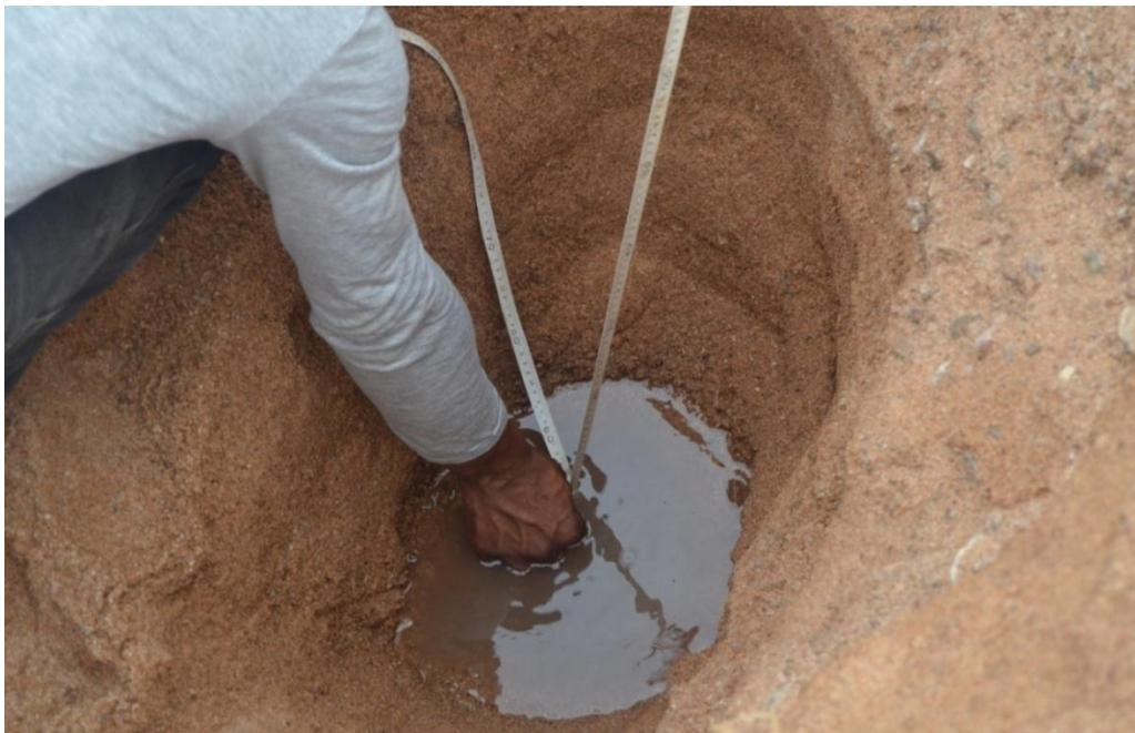
Figure 15: Measuring depth to water level
