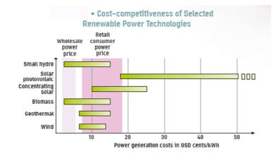
Figure 12: Comparative per unit cost of RE-power generation, and the current wholesale and retail per unit power price.
