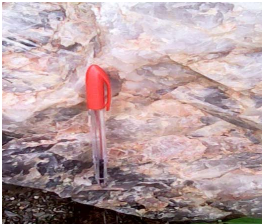
Figure 2. (a) The simplified geology map of the study area showing road network and some geological features; (b) A massive outcrop of quartzite with joints which is one of geological feature in the study area.
